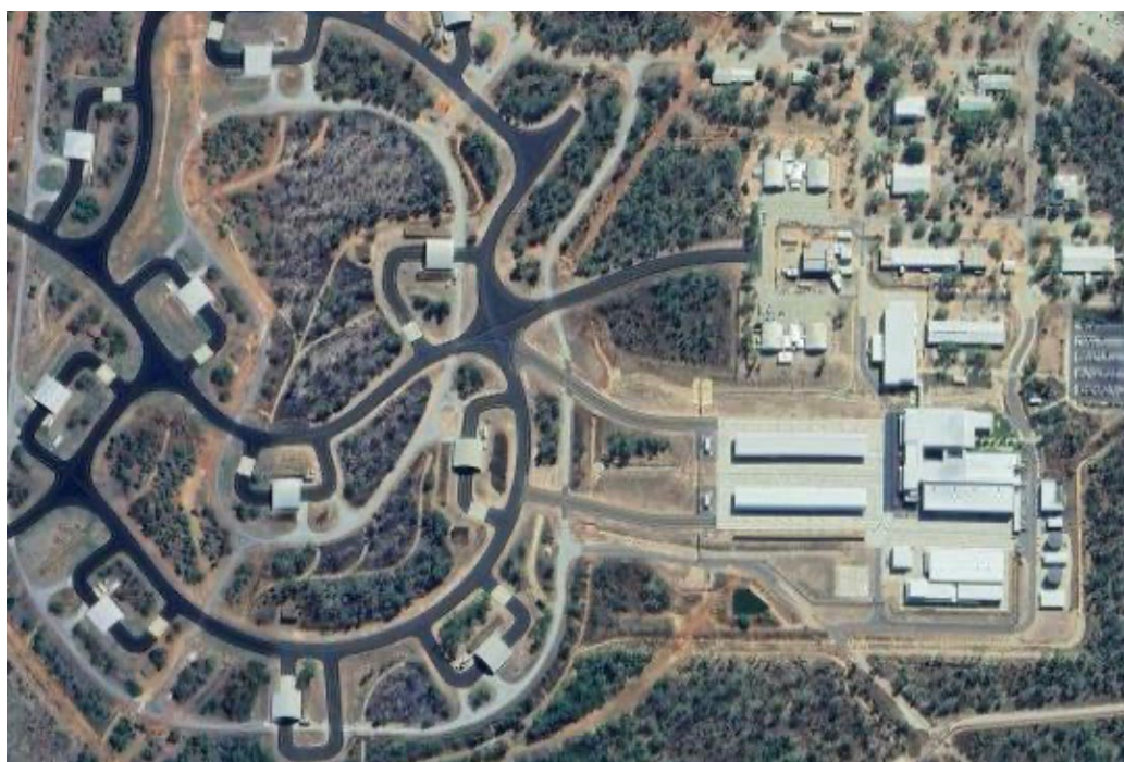
Figure 2: Satellite photograph of RAAF Tindal, showing dispersed aircraft operational areas to the left of the image and consolidated aircraft operational areas to the right. 14
