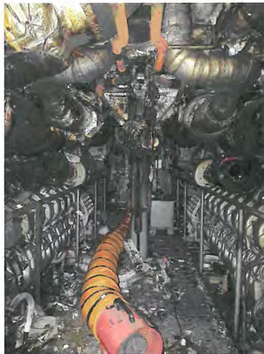
Figure 9: Between both engines looking aftwards. Significant damage to the lagging as well as the deck covered is bits of lagging. Near the king post the light fitting is being held up by its wires.
