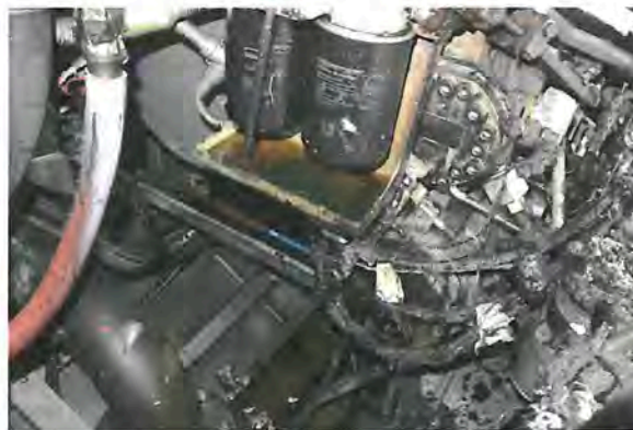
Figure 13: Pool of diesel below two filters of engine one.
