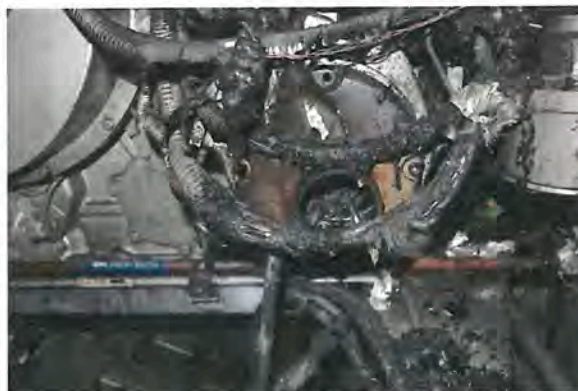
Figure 5: Alternator fitted to engine one, impacted by combustion
