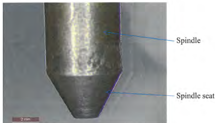
Figure 3 Steel spindle seat and minor corrosion above sealing surface
