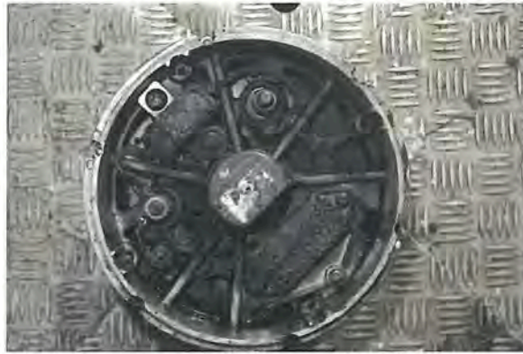
Figure 6: Removed alternator with signs of fuel ingress and combustion
