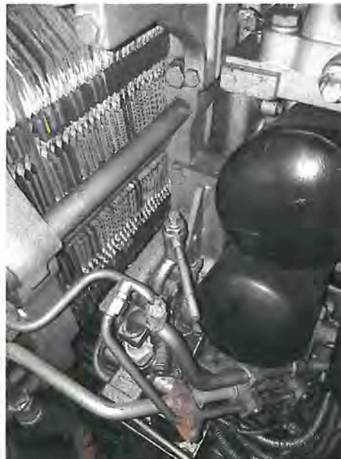
Figure 3: Bleed off assembly for Engine 2, showing the nominal condition.
