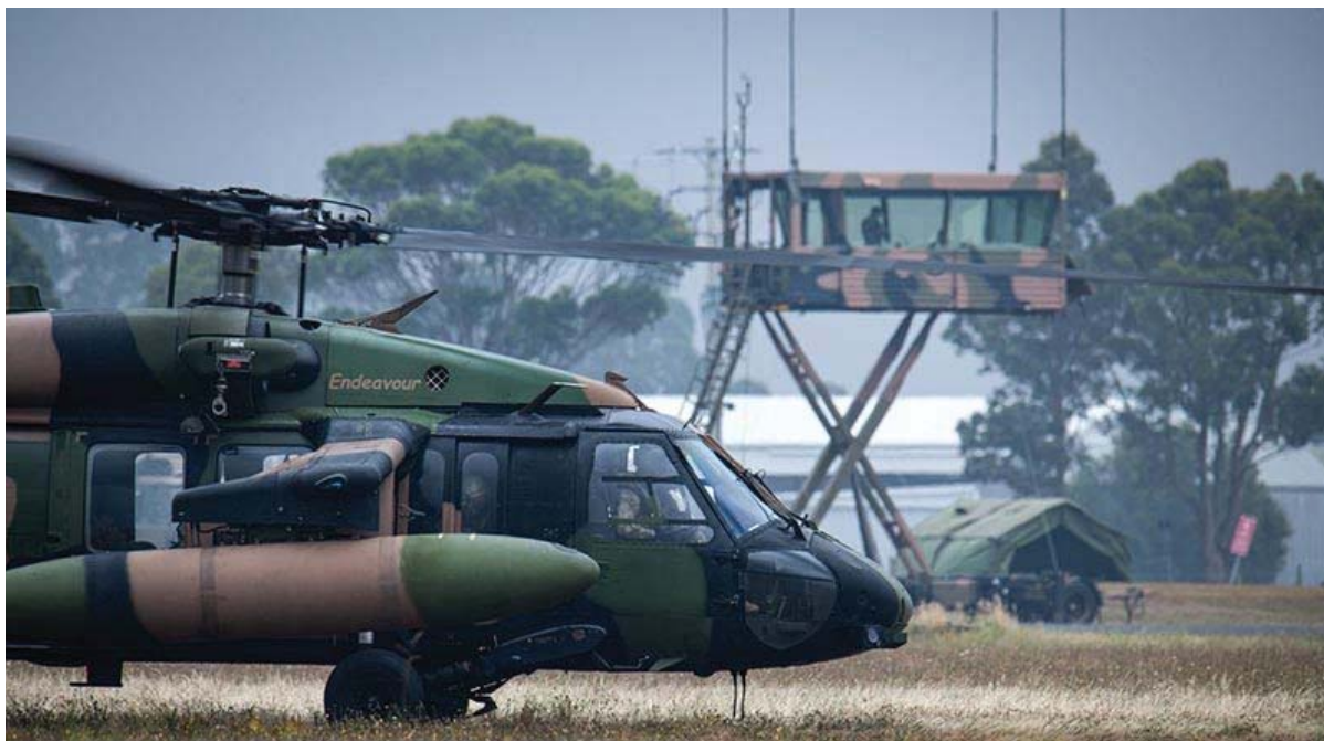
Image: Transportable Air Operations Tower (TAOT). The TAOT is a deployable system operated by 44WG Deployable Air Traffic Control Flight (DATF) that can provide Ground-Ground, Air-Ground-Air voice communications and data exchanges using landlines and radios. The TAOT is able to provide air traffic services. The TAOT provides localised airspace information to airspace users and other agencies when deployed to Bairnsdale, Victoria in support of Operation 'Bushfire Assist' in Jan 2020
