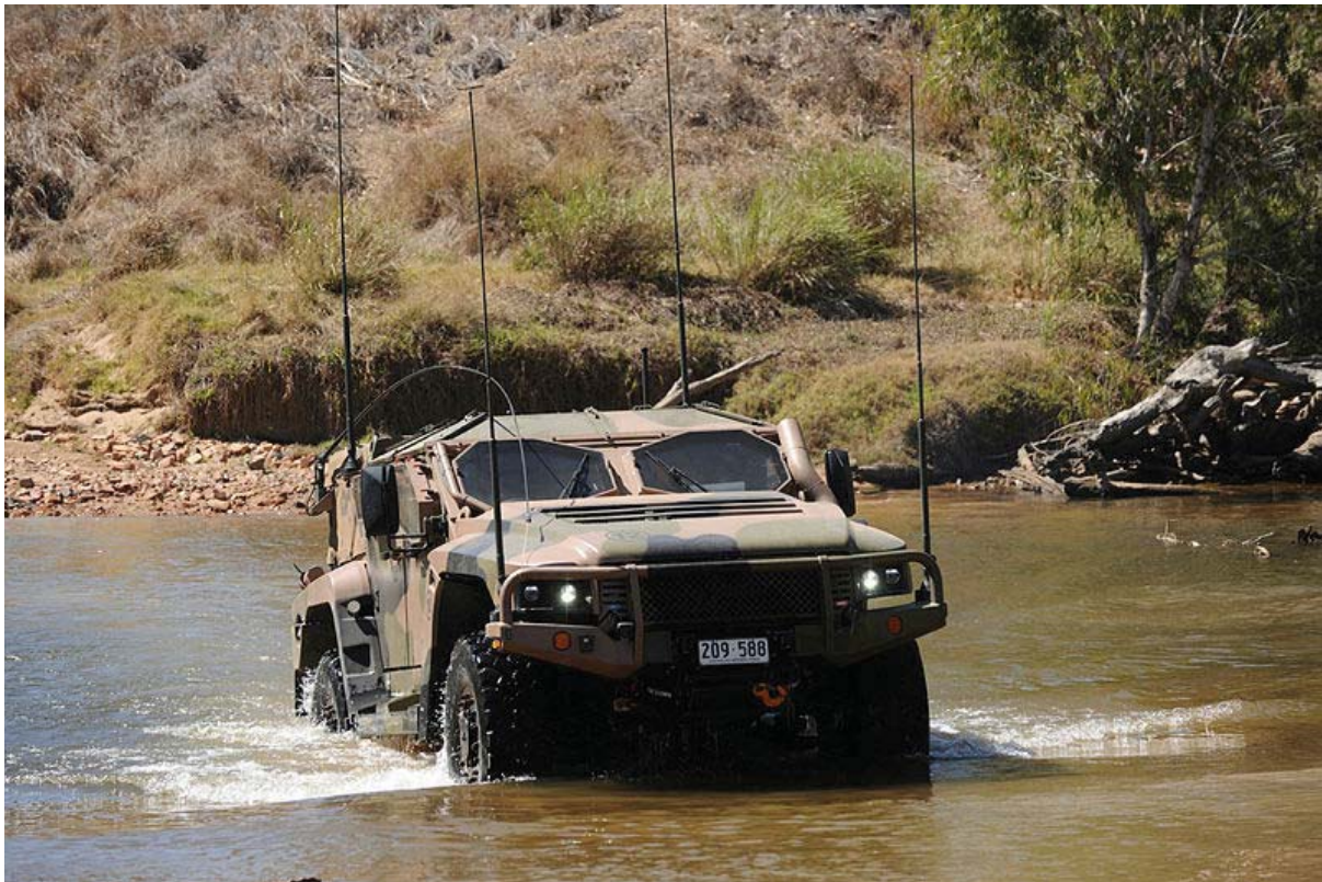
Image: Hawkei undergoing water fording testing.
