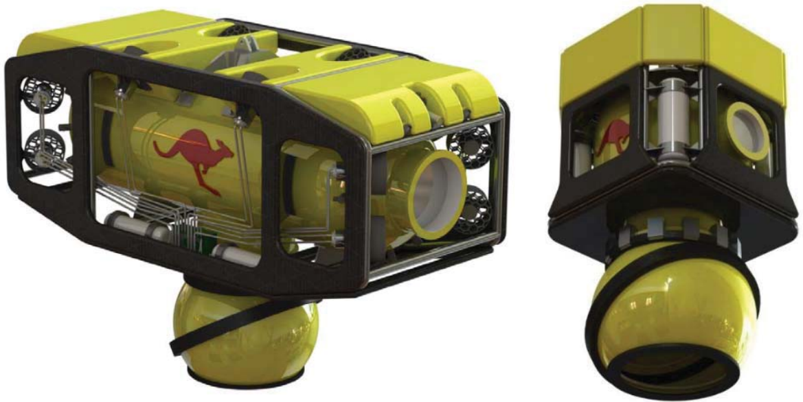
Image: An image of the Remotely Operated Rescue Vehicle and Shallow Water Rescue – Diving Bell that forms part of the Submarine Escape Rescue and Abandonment System.
