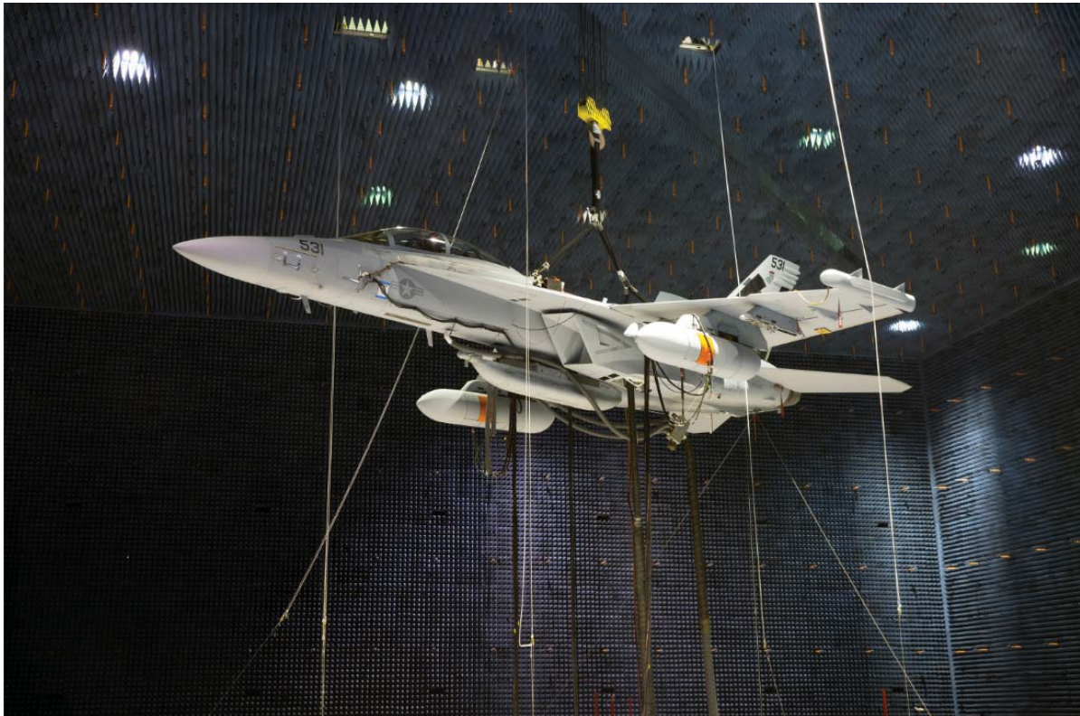
Image: Growler fitted with NGJ-MB for testing in anechoic chamber, 19 March 2020 (supplied by US Navy).
