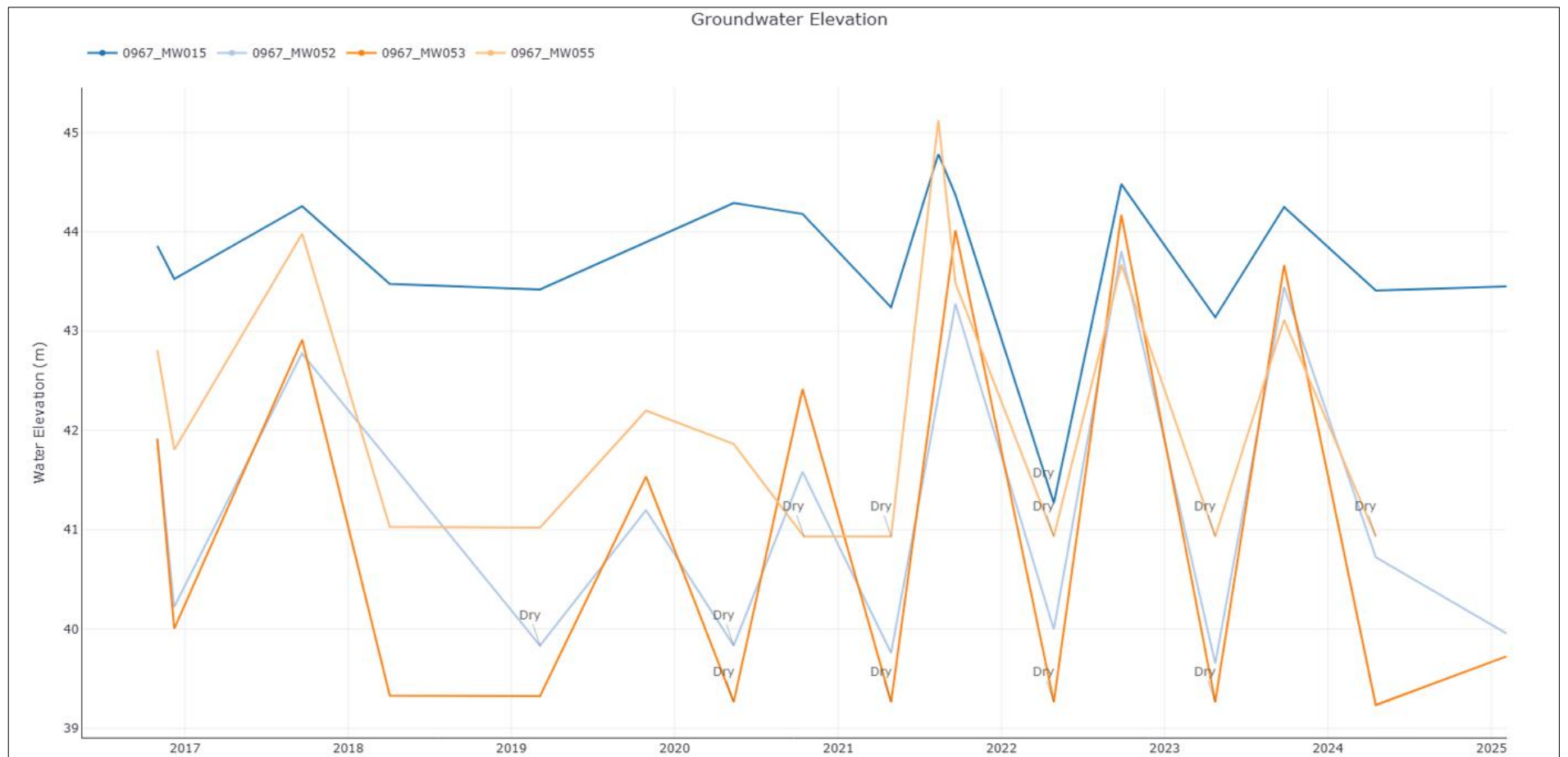
Graph G.1 Groundwater elevation - Perched aquifer
