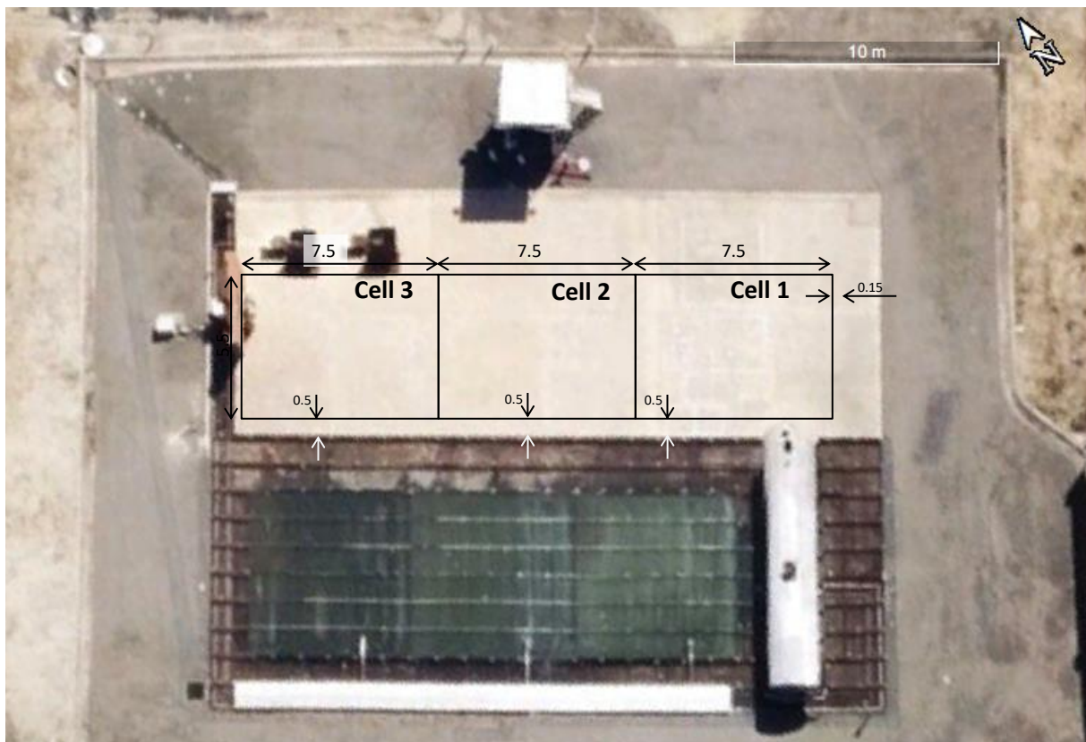
Figure 3.10 Sealed and unsealed areas of the concrete pad – Cell 1 = Epoxy/Polyaspartic, Cell 2 = Control, Cell 3 = Lithium densifier/Polyaspartic. Dimensions in metres.
