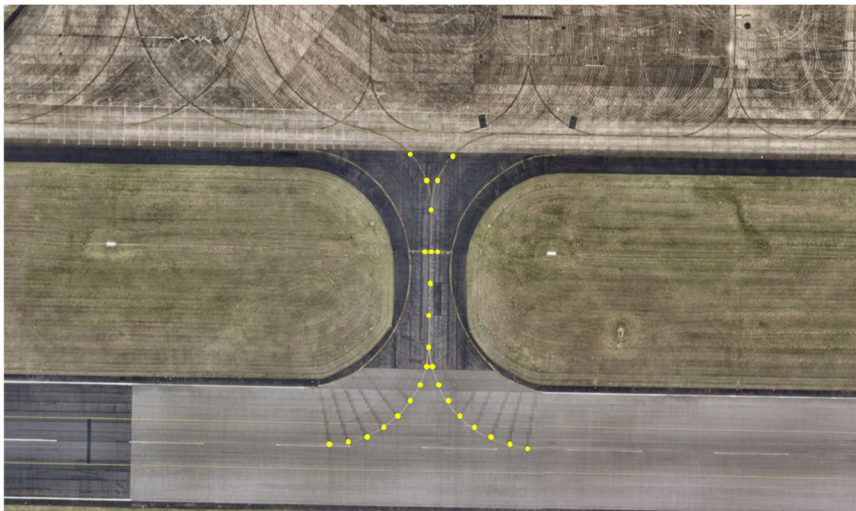
Figure 6 - Survey, isolate inset lighting, removal of lights/cans & temporary lighting install
