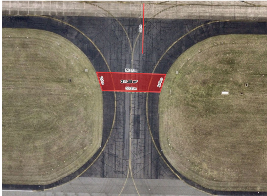
Figure 8 - Profile 100mm Asphalt from Hold Position lights to Taxiway Z (plan view)
