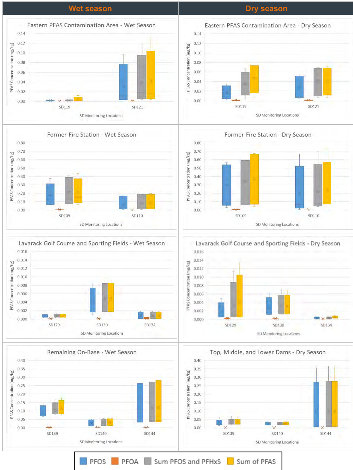
Figure D.3 Seasonal sediment PFAS concentrations in on-base and off-base locations in the Management Area (2017 to 2024)
