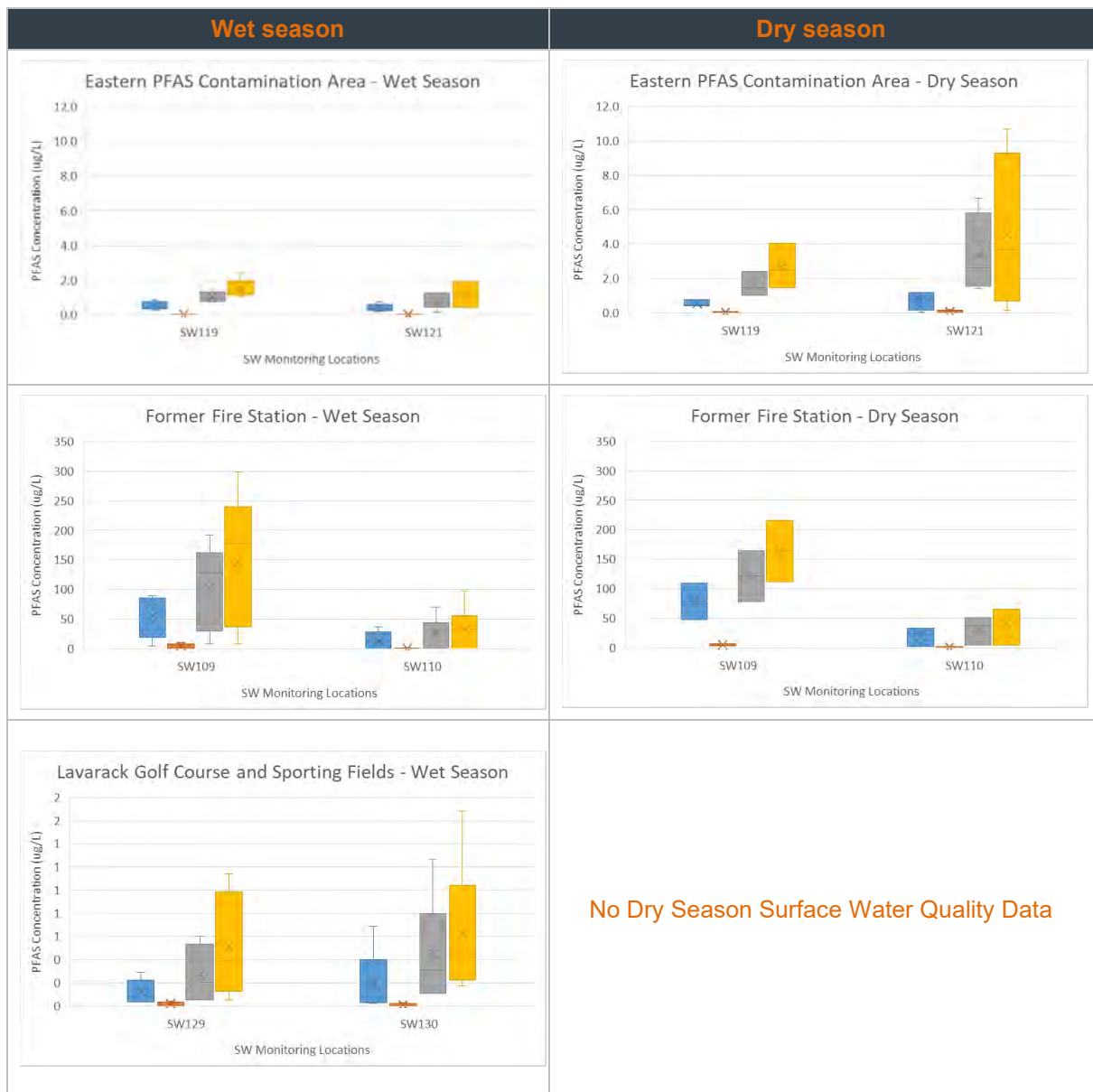
Figure D.2 Seasonal surface water PFAS concentrations in on-base and off-base locations in the Management Area (2017 to 2024)
