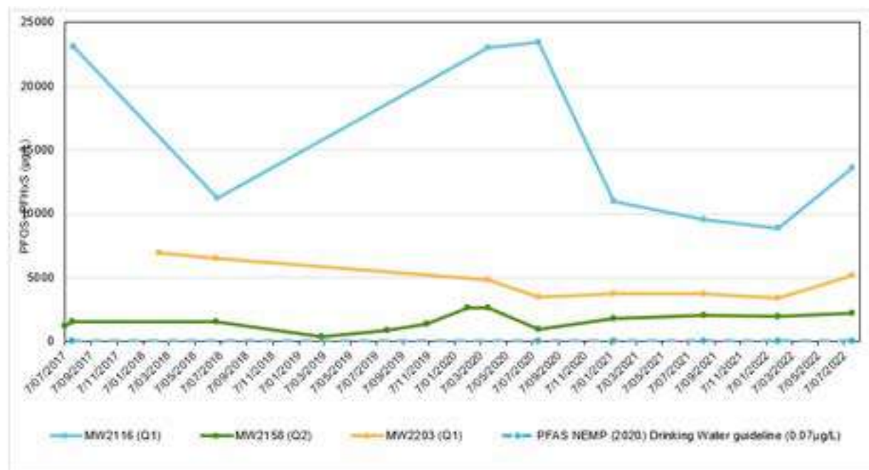
Figure 12 Q1 and Q2 monitoring wells PFOS+PFHxS concentration trends at source areas P9 and P15A/B, P11, P16 and P21 (above 1000 µg/L)*
