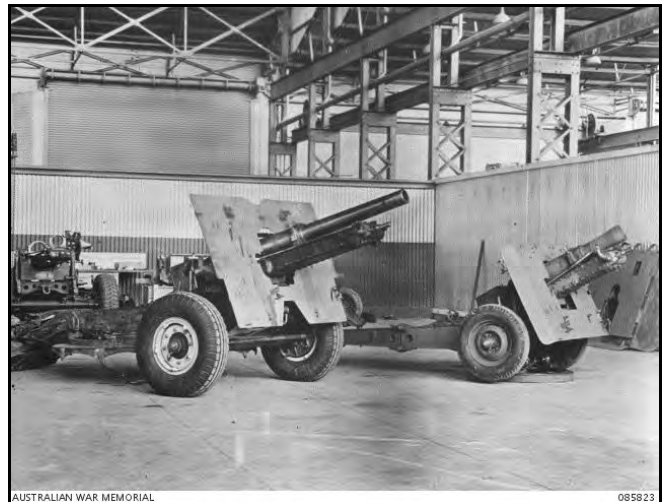
Figure 3 - Standard (left) and Short (right) 25-pounders. This is the prototype, which was fitted with a gun shield that was later removed (AWM ID 085823)
