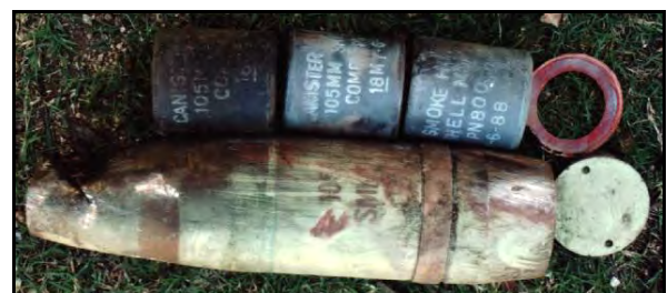
Figure 5 - Expended 105mm Smoke showing expended smoke pots.
