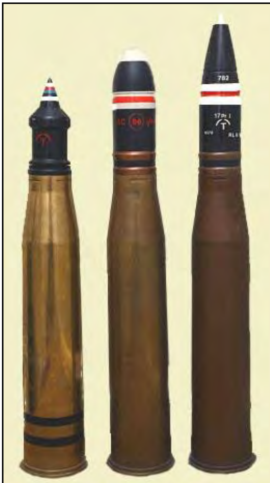
Figure 3 - Example 17 pr complete munitions (LtoR): APDS, APC, APCBC
