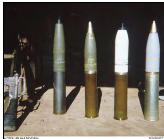
Figure 3 - Various 105mm projectiles used during the Vietnam War. LtoR: Anti Personnel (Flechette); High Explosive; Parachute Flare, Smoke (WP) (AWM ID P01636.017)
