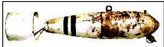
Figure 4 - Recovered UK/Commonwealth Practice Bomb
