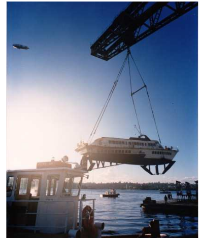
Figure 2.30 The HHC lifting the hydrofoil out of the water for repairs. (Source: Naval Historical Society)
