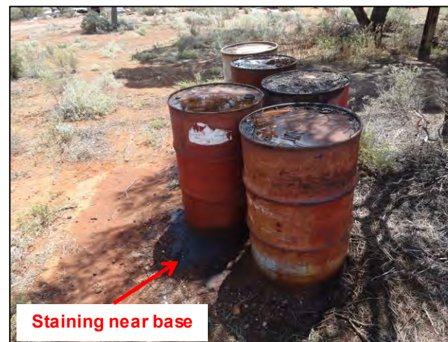
Plate 2: Evidence of surface soil staining around base of drums
