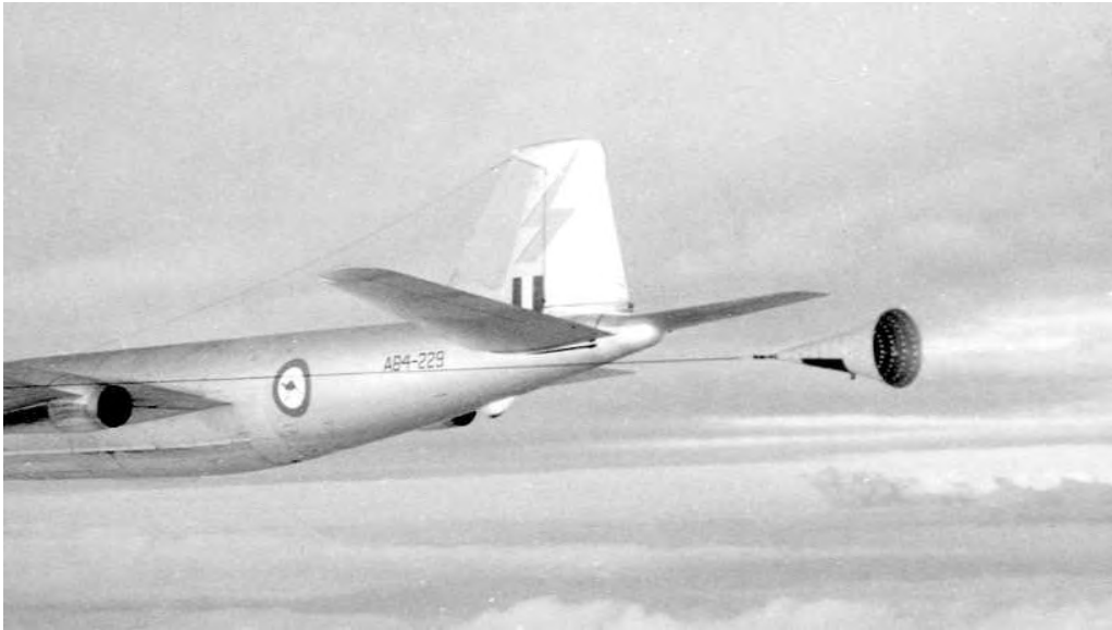
Plate 23 Canberra bomber trailing a drone used to collect atomic dust samples (Source: Amberley History n.d. 101)
