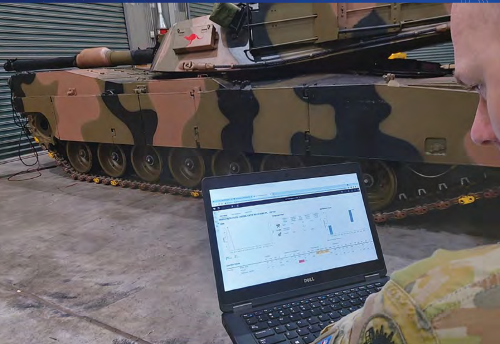
A soldier using the Vulcan Oil Condition Monitoring dashboard at the Army School of Electrical and Mechanical Engineering, 2021. Photo Credit: Nick Draper.
