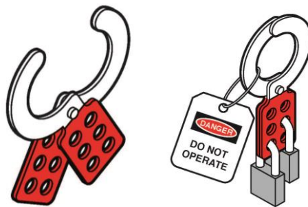
Figure 1 Example of tag and lockout with the padlocks of two workers.
