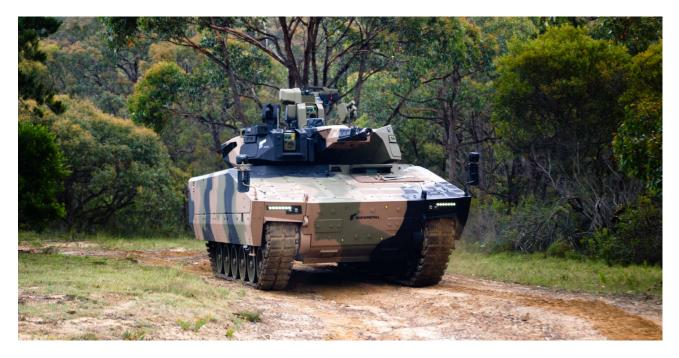
The RMA Vehicles are fitted with a LANCE turret and the IFV Role kit, accommodating a Crew of 3 and 6 Dismounts. LYNX features a number of offensive capabilities, such as direct fire and indirect fire weapons, Counter UAS capability (direct shoot-down through Air Burst Munitions), defensive enablers via passive and active protection systems, and a cutting edge C4ISR fitout.
