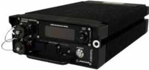
The TSR is a rugged hardware computing platform that hosts the IP networking, routing, video, voice and data services for deployment communications networks. The TSR uses an industry standard and upgradeable Computer on Module (COMe), with the current model providing a Gen6 Intel Xeon processor and 16GB of RAM. Future TSR models will support the latest Intel Processors.
