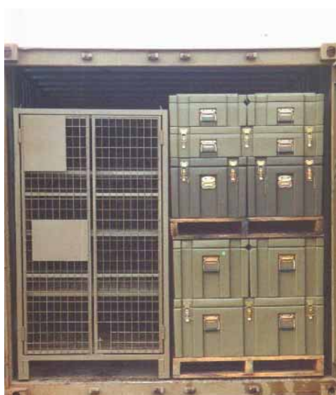
Figure 2a. Cube utilisation (Under-utilised)
