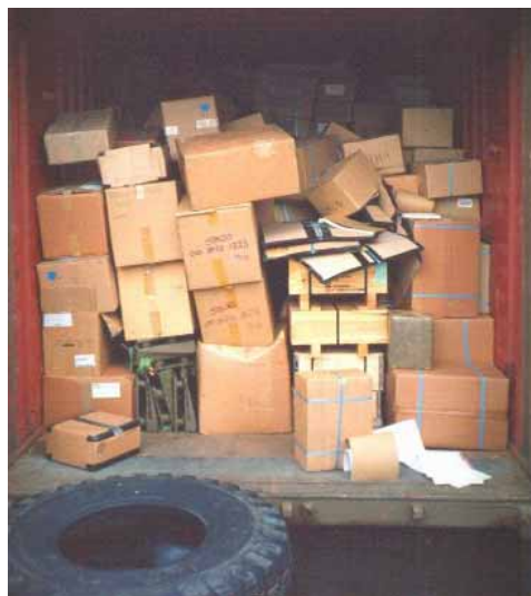
Figure 1b. Unsatisfactory method of stuffing cardboard cartons
