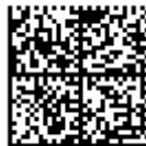
Figure 21 - Example Data Matrix Bar Code
