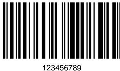
Figure 22 - Example Code 128 Bar Code
