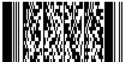
Figure 23 - Example PDF417 Bar Code
