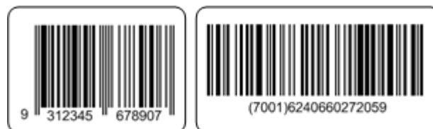
Figure 1 - Example EAN/UPC Bar Code with NSN encoded in a GS1-128 Bar Code
