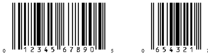
Figure 17 - Example UPC-A and UPC-E Bar Codes
