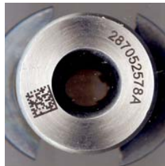
Figure 5 - Laser Etch UID Mark (with Serial Number as HRI)
