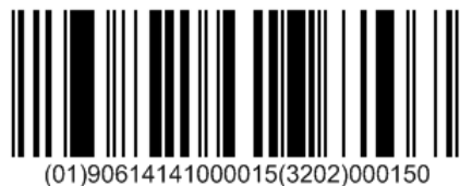
Figure 18 - Example GS1 DataBar Expanded
