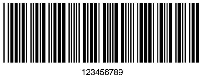
Figure 24 - Example Code 39 Bar Code
