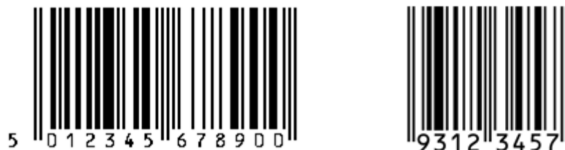
Figure 16 - Example EAN-13 and EAN-8 Bar Codes
