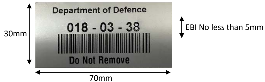
Figure 3: Example of Space (Room) Label Format
