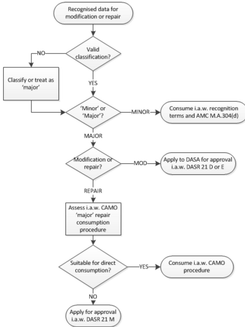
**Figure 1 – Treatment of approved data for modifications and repairs accessed through recognition**
