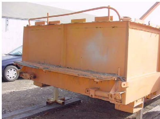
Rear view (timber ledge needs replacing)
