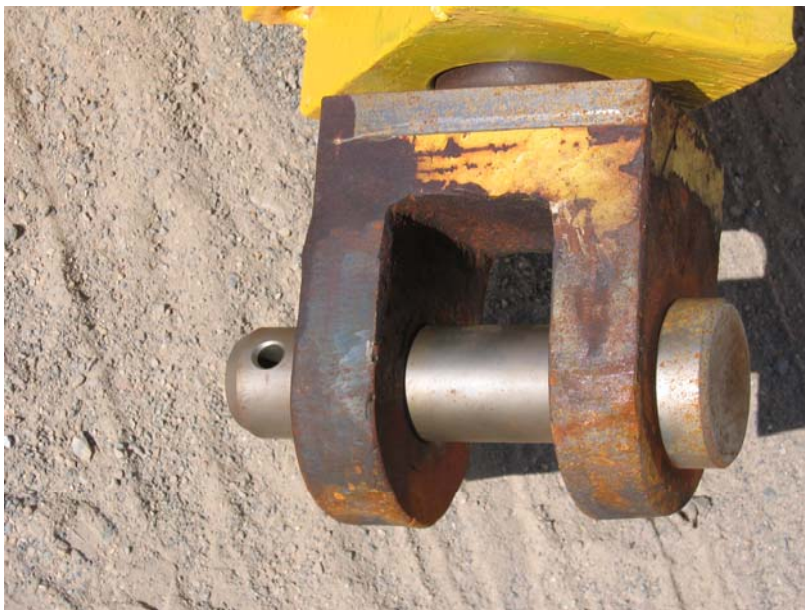
Photograph 8. Replaced hardened steel draw-bar pin.
