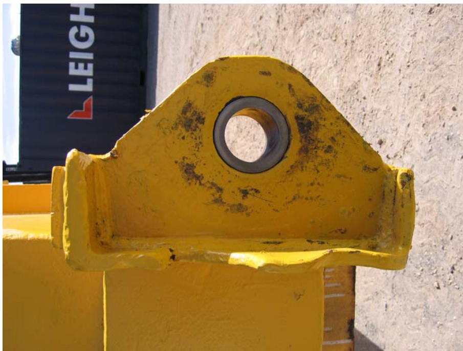
Photo 2. Replaced hardened steel bushes.
