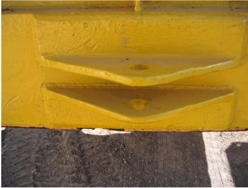
Photograph 7. New rear flanges.
