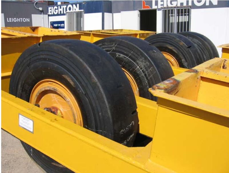
Figure 10. Bridgestone 16.00-25 32 Ply YS2 tyres fitted to roller.
