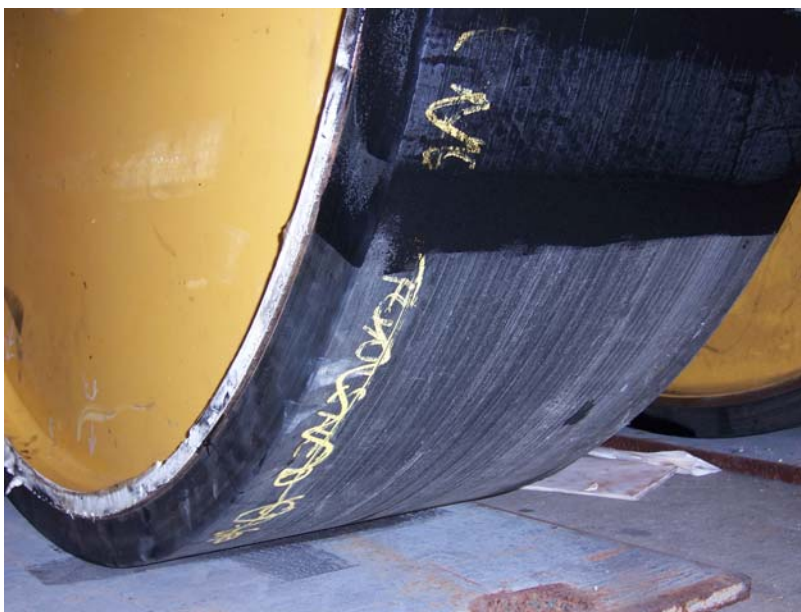
Figure 8. Solid steel wheels with urethane tyre.
