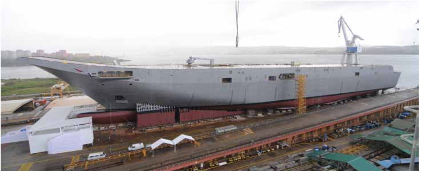
A side-on view of the LHD hull launched in Spain.
