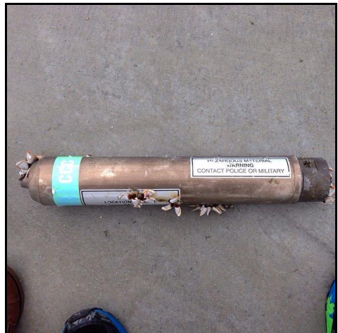
Figure 5 - Marine Marker C2A2 (similar to Mk 25) washed ashore onto beach
