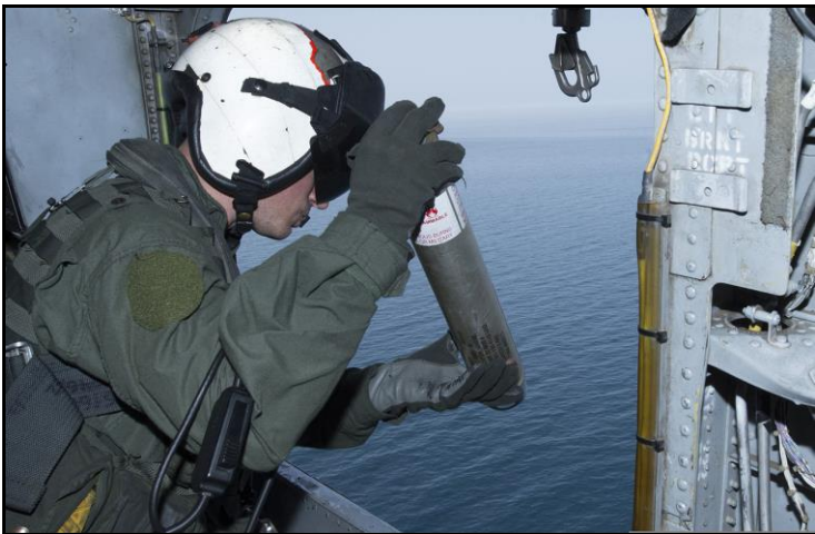
Figure 2 - US Navy Aircrew deploys a MK-25 marine location marker (Public domain photograph from defenseimagery.mil)
