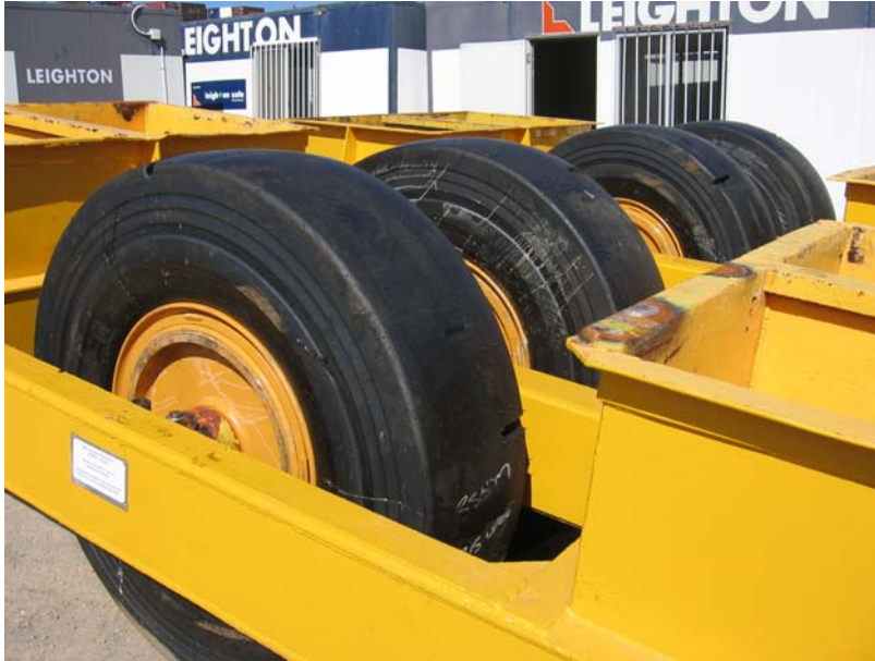
Photograph 6. New Bridgestone 16.00-25 32 Ply YS2 tyres.
