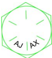
Figure 2. Pneumatic tyred roller wheel nut, note radial marks denoting Grade 5 Bolt.
