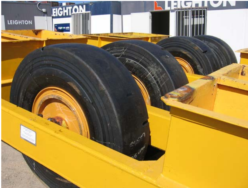
Figure 10. Bridgestone 16.00-25 32 Ply YS2 tyres fitted to roller.
