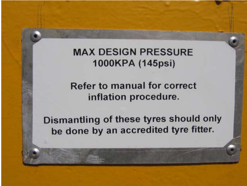
Photograph 10. New tyre inflation instruction plate.
