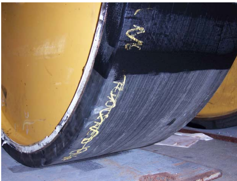
Figure 8. Solid steel wheels with urethane tyre.
