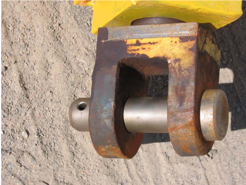
Photograph 8. Replaced hardened steel draw-bar pin.
