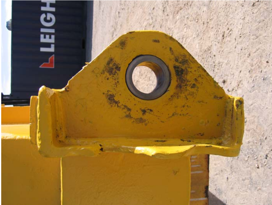
Photograph 2. Replaced hardened steel bushes.
